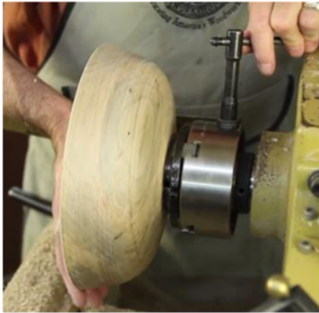
Scroll chuck being tightened to bowl for hollowing
