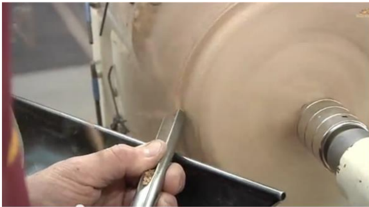
Bowl Turning Gouge being used to round outside of bowl “with-the-grain”. (Using under-hand grip with thumb holding gouge down onto tool rest and tool tip “riding the bevel”)
