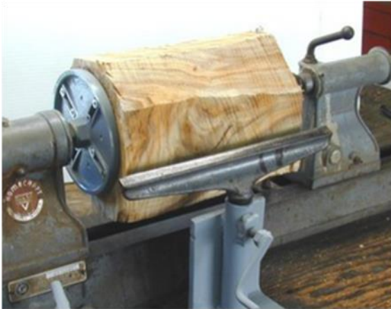
Work being held by a combination of face plate and revolving dead centre
